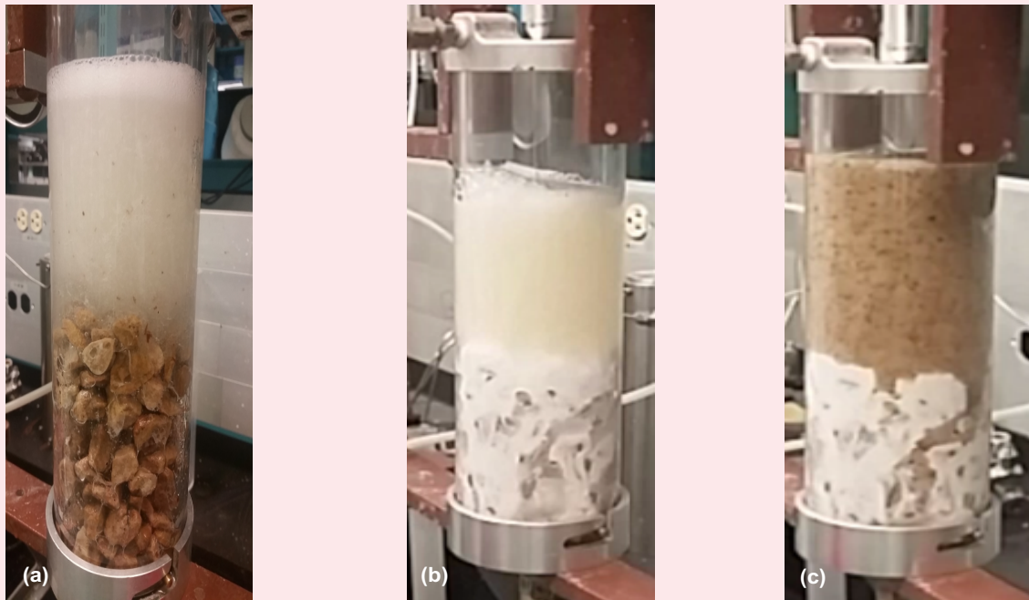
Fig. 5 The LPLT test using pebble bed for (a) polysweep, (b) polysweep system, and (c) polysweep plus date tree roach root fibers.
