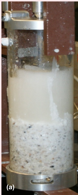
Fig. 4 The LPLT test conducted using carbonate bed material for (a) polysweep, (b) Soluseal, and (c) stoploss.
