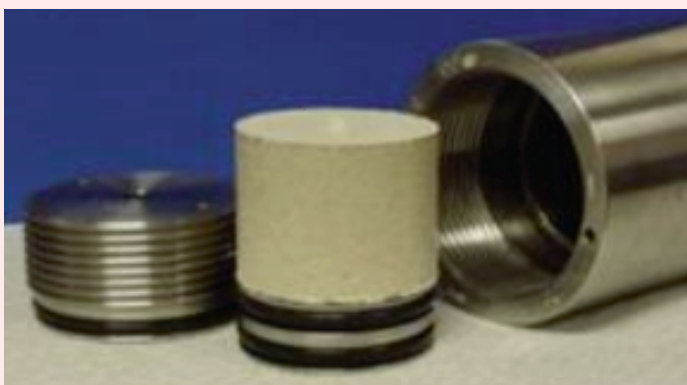
Fig. 1 High strength plug from a laboratory test on the pressure-activated LCM pill.
